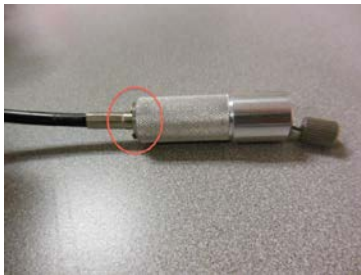
Pre-2011 Float 30 No Upgrade Needed
